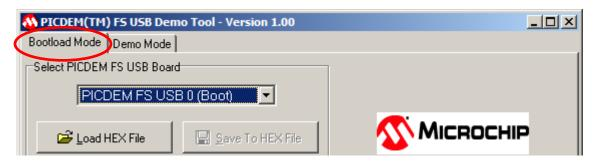
7. In the Select PICDEM FS USB Board, select "PICDEM FS USB 0 (Boot)" from the pull-down menu. If there are no options showing, make sure that the shuttle is connected to the computer.
